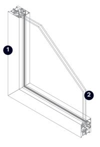
1 Aluminium profile with thermal break
